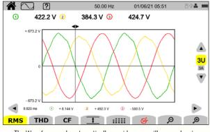
The Waveform mode automatically provides an oscillogram showing the voltage and/or current waveforms.
